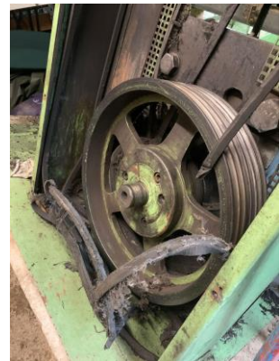
The gearbox drivebelt shredded at the beginning of October
