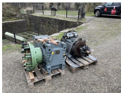
Gearbox (left) and generator
